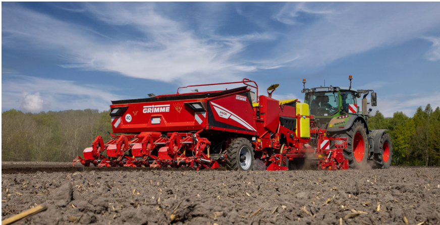
Bucket laying machine for laying potatoes
