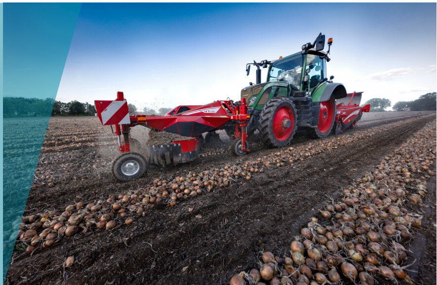
Onion haulm beater for efficient haulm separation
